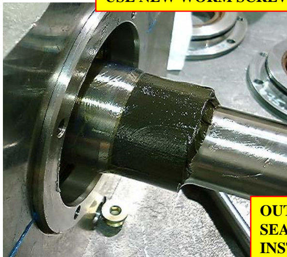
WITH BOOT INSTALLED AND FIRMLY SEATED USE NEW WORM SCREW CLAMPS AND TIGHTEN
